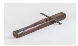
The *Tiangong Kaiwu* also records the basic variations of the plane, including the long plane (*zhangbao* 長包). "Long ones," like the Western jointing plane, as opposed to the shorter and more common jack or scrub plane, were used to surface long, straight edges that could be well matched, and were thus indispensable for making water-tight barrel staves (cf. fig. 31). Using the plane in a fixed and inverted position was an innovation that foretells the modern jointer. Split timbers are
