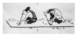
Because the adze leaves a scooped surface typical of roughly hewn timber, ancient woodworkers attained a further level of refinement by using a long-handled, spear-like paring knife (*si* 鐁). Excavations of ancient sites throughout China indicate that such a tool was in common use over a widespread area. The long, narrow blade is shaped like a willow leaf, and is sharpened on both sides;
