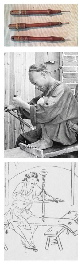
with a centering point and acutely angled cutting faces. The one-*fen* bit has a three-sided point, and a spiral groove is hand filed up its entire length to facilitate chip removal. Although made of hand-wrought iron, both of these bits are patterned after modern bits that spin in only one direction. The smallest bit of the three has three flat sides that come sharply to a point, and is patterned after the "twisting awl."
