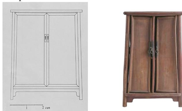
The cupboard is 5.05 *chi* (151.5 cm) high, 1.65 *chi* (49.5 cm) deep, and 4.4 *chi* (132 cm) wide. (The space between) the two (front) posts is divided equally. Each post is .16 wide x .14 *chi* thick. The bottom rail is .14 wide x .13 *chi* thick; the top rail is .14 wide x .12 *chi* thick. The
