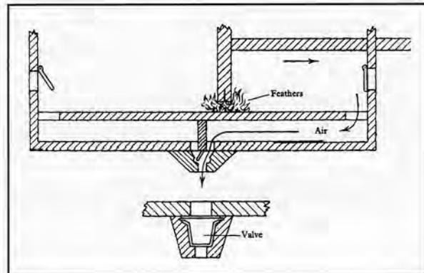
Fig. 8, left. Drawing of a section through the double-acting bellows. After Needham IV, fig. 427c, d.
